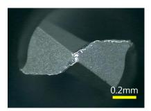
Tool after drilling 20 holes
