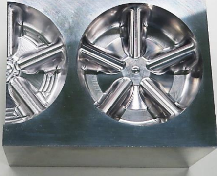
Work after milling
