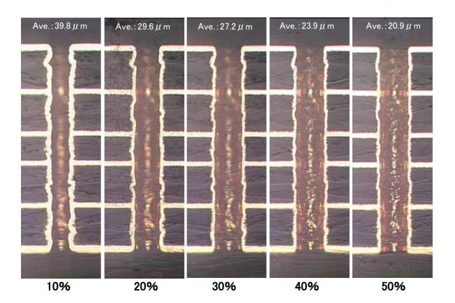
The hole wall roughness on the cross section was Ave.:39.8  $\mu$  m at 10%, but it decreased Ave.:20.9  $\mu$  m at 50%. Cross-section pieces should be made carefully.
