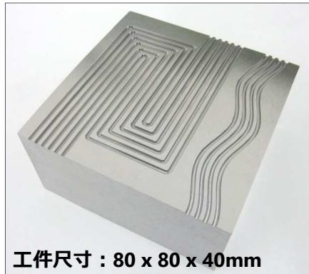
2刃避空型圆角刀 **CBN-LRF  $\phi 1 \times CR0.1 \times L1$**
