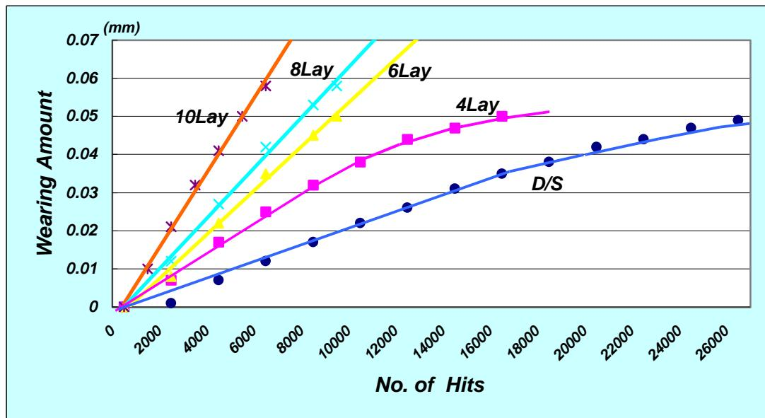
Note : The thickness of the 8 layers board is 1.2 mm. All other boards are 1.6 mm thick.
