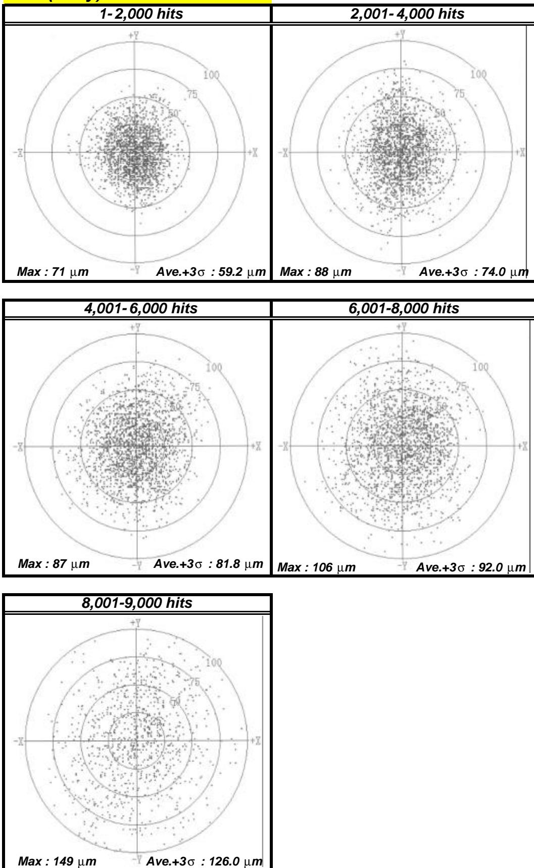
REMARK : Measured on the back side of the bottom panel only.
