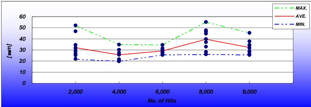
Remark : Measured after desmearing treatment and on the top panel only.
