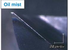
When using oil mist, the tool wear become smaller than water soluble.
