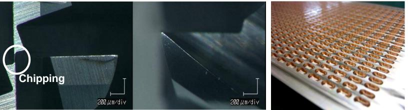
Although 1,600 slits were milled, the tool wear were small. Only the small chipping was in the center of bottom edge. There is no burr on the workpiece.
